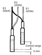
Note: 1. When the distance between E1 and E3 exceeds 1 m for supplying purified city water, for example, locate a second E3 within 200 mm of E1.
