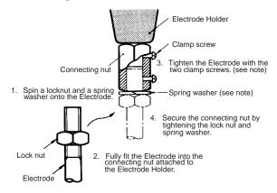
Note: Clamp screw and spring washer are not provided for the BS-1T Electrode Holder (titanium, hastelloy B, or hastelloy C).
